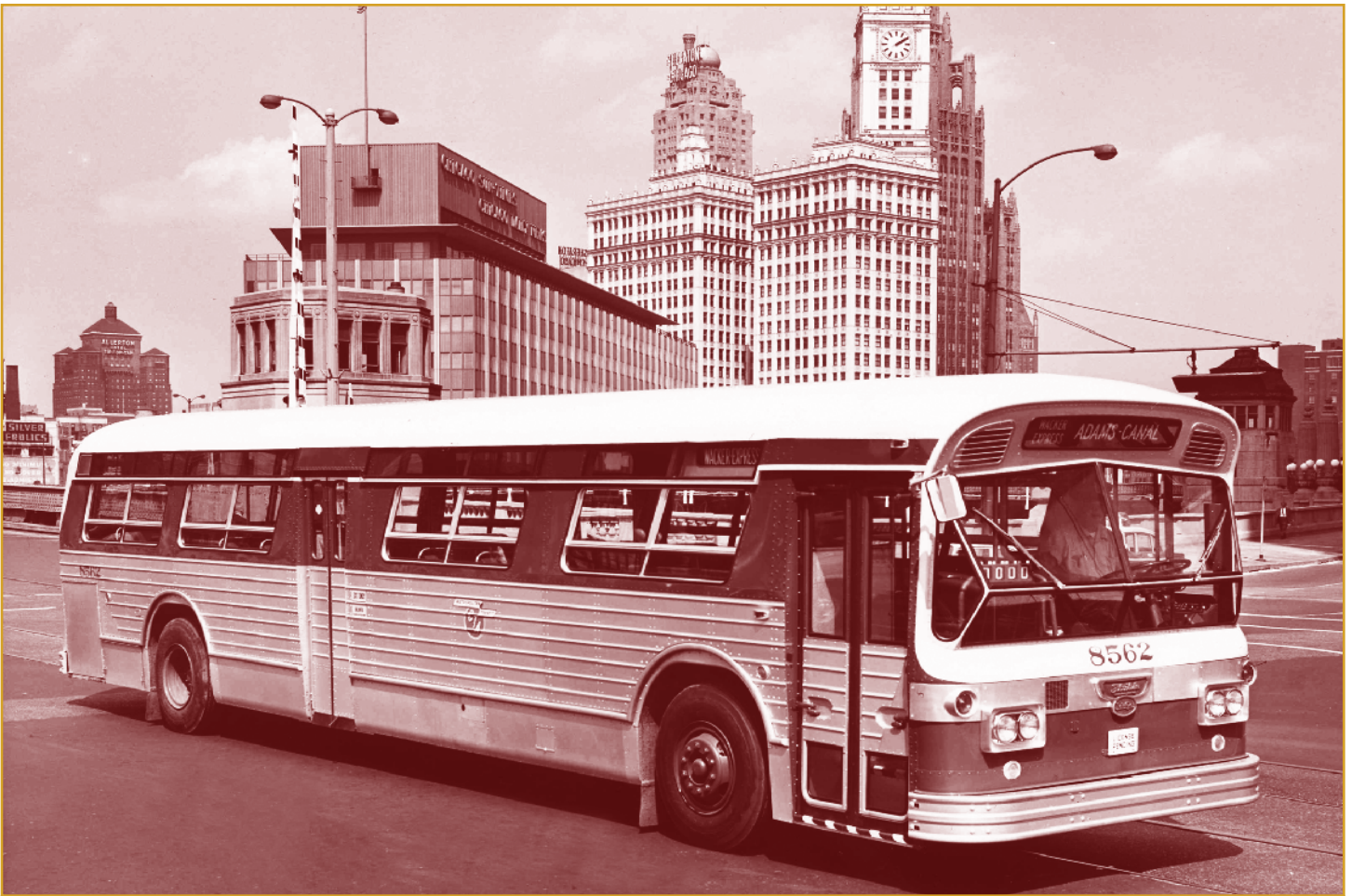
CTA "New Look" bus #8562, built by the Flexible Company in 1961, has just arrived from the factory and is crossing Wacker Drive at the Chicago River. The CTA was in the process of modernizing and enlarging its bus fleet, having completed the last of the streetcar-to-bus route conversions just a few years earlier. The 8500-series buses were used until 1975.
