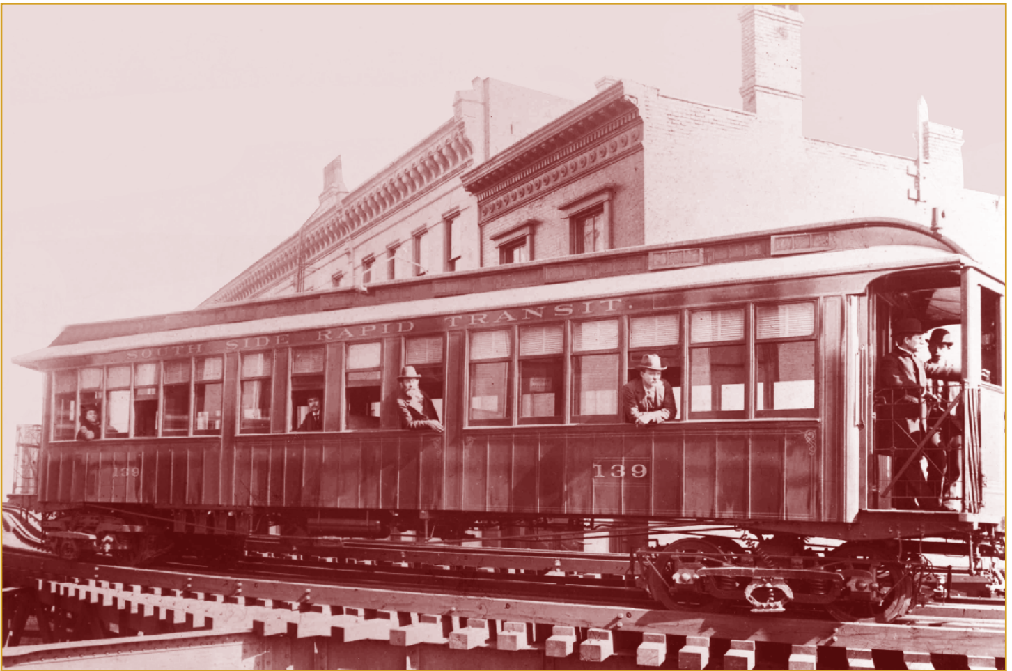
South Side Rapid Transit car #139 is seen heading southbound at the Harrison curve on the South Side Elevated in this 1898 photo. The car is testing the new electric traction equipment planned for converting the South Side 'L' from steam to electric power. Frank Sprague, the man charged with overseeing the work, is seen in the vestibule of the front car, in discussion with the motorman.
