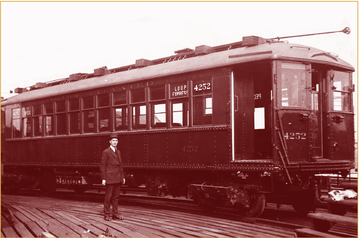
It is 1923 and Chicago Elevated Railways car #4252 has just been received from its builder, Cincinnati Car Company. The 4251-4455 group of 4000-series cars featured the newest amenities of the time, including plush seats and electric fans for the passengers' comfort, and new shaded lighting.
