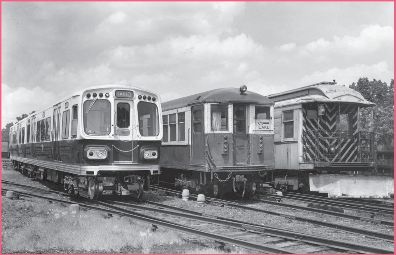
Three generations of rapid transit cars that served the Lake Street 'L' are seen lined up in Hamlin Yard on June 19, 1964 – 1964-built “New Look” High-Performance cars 2011-2012 (left), 1915-vintage “Baldie” car 4145 (center), and open platform wooden car 3146 (right).
