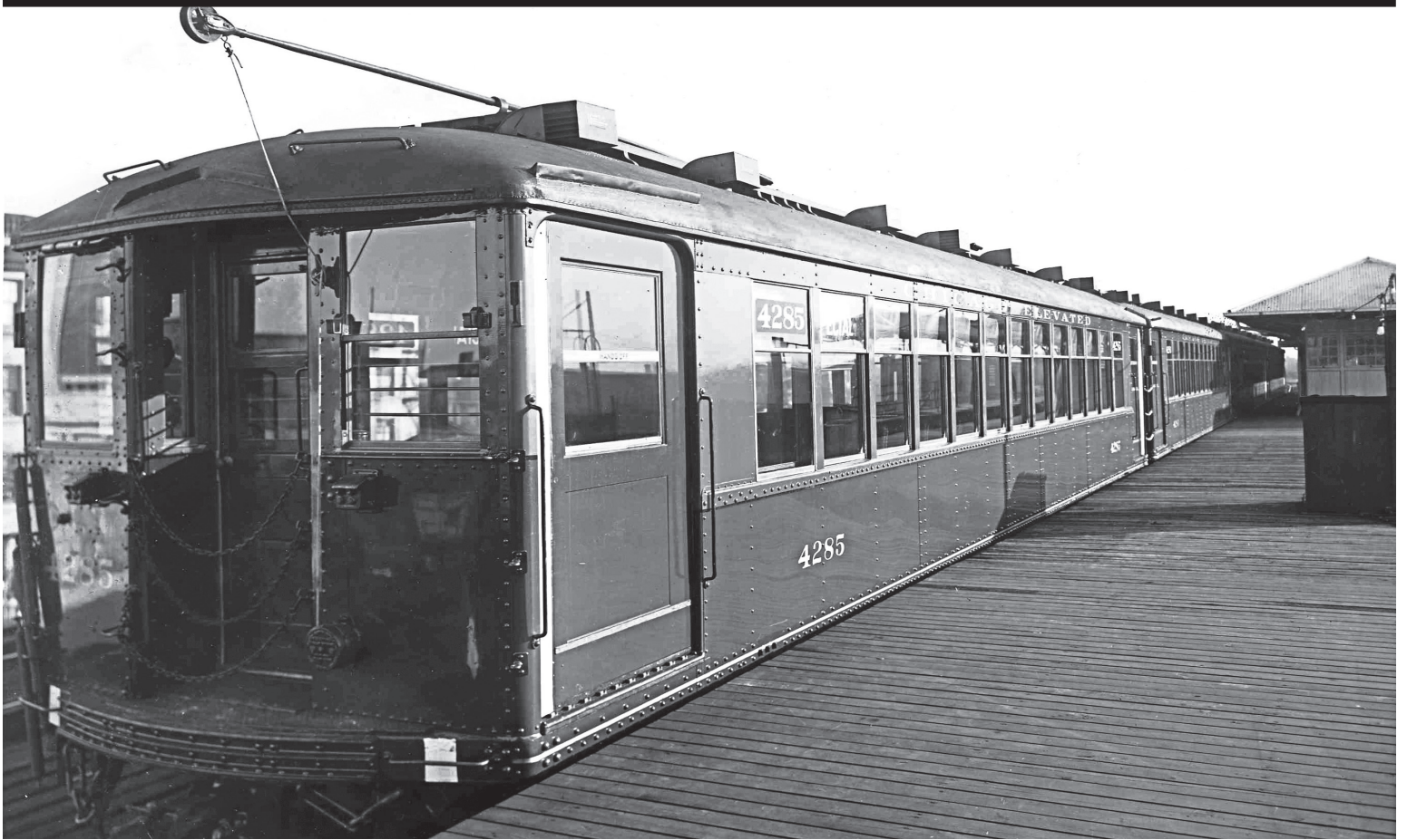
A four-car train of 4000-series rapid transit cars, headed by car #4285, occupies the northbound express track at the Wilson station on the north main line of today's Red Line. Newly arrived from the Cincinnati Car Company in 1922, the cars are resplendent in their fresh paint scheme of a green body and burnt orange through the windows, with a salmon-colored roof. Three orders of these cars were placed between 1922 and 1924, ultimately totaling 205 cars. The cars shown in the photo were built for the Chicago Elevated Railways, a voluntary association of the various independent rapid transit companies that existed in the early days of Chicago's transit history, prior to becoming part of the Chicago Transit Authority beginning October 1, 1947. A select number of 4000-series rapid cars have been preserved, including cars #4271-4272 that remain on CTA property and are operated for various special occasions. In addition, cars #4420 and #4453 are at the East Troy Trolley Museum in East Troy, WI; cars #4103, #4288, and #4451 are at the Fox River Trolley Museum in South Elgin, IL; and cars #4146, #4290, #4321, #4410, and #4412 are preserved at the Illinois Railway Museum in Union, IL.
