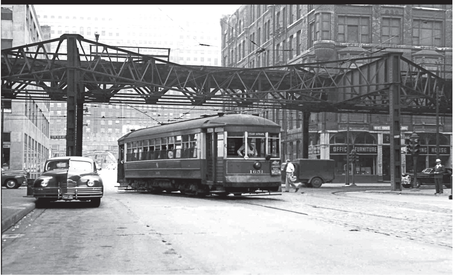
CTA streetcar #1651, signed for the Division-Downtown route and still in the red and cream livery of its predecessor company, the Chicago Surface Lines, is turning south from Lake Street onto Franklin, carrying its load of passengers into the Loop. This series of cars, nicknamed "Turtlebacks" due to the uniquely shaped arched roof suggestive of a turtle shell, were built between 1911 and 1912 by the Chicago Railways, one of the independent streetcar companies absorbed into the Chicago Surface Lines two years later. They operated on various routes on the north and west sides, with the last of these cars being retired in 1950. (Mike Charnota collection)
