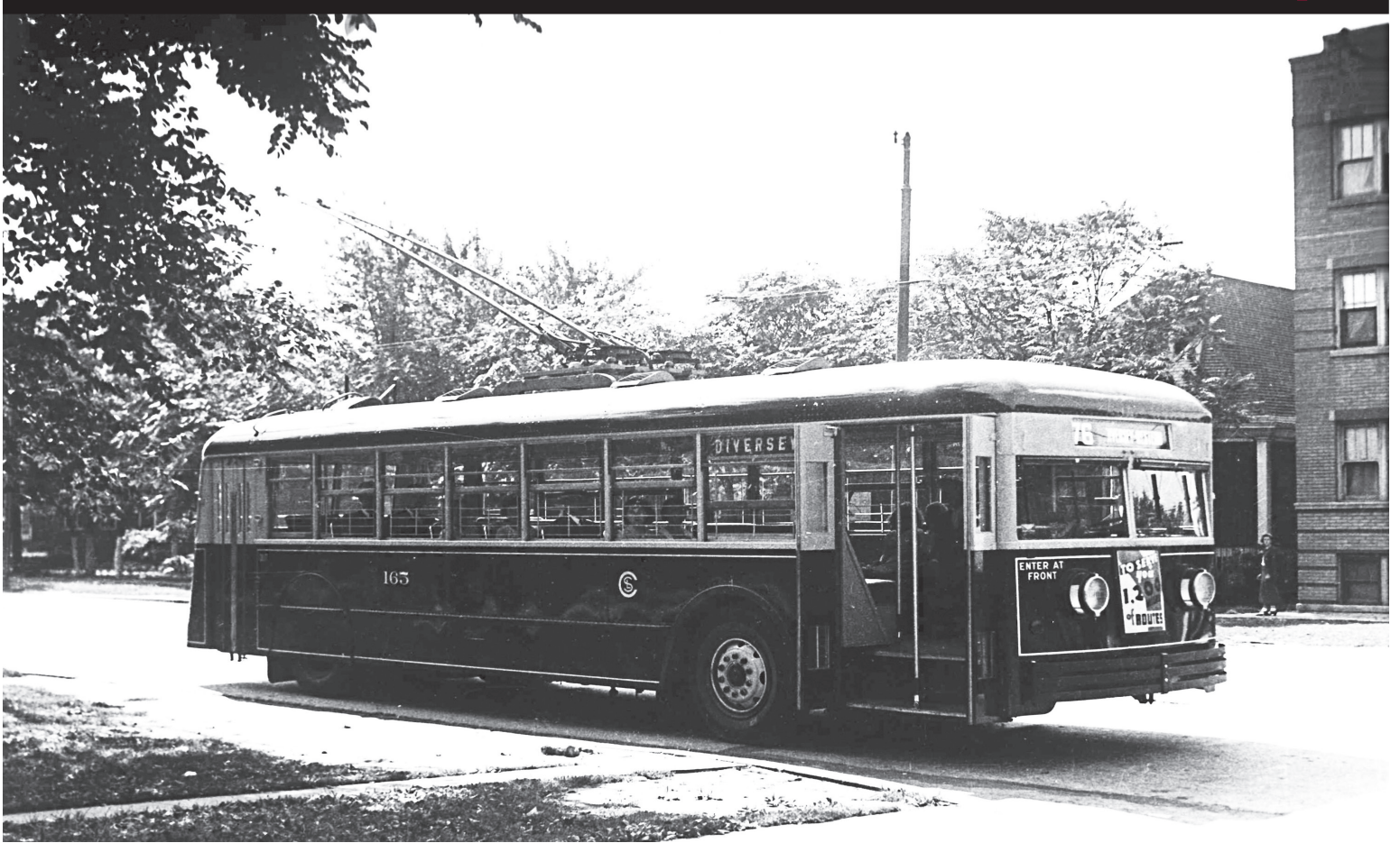
Chicago Surface Lines (CSL) trolley bus #165, signed for the #76 Diversey route, is seen at Central and Wabansia. Built by the Pullman-Standard Car Company in 1935, with a seating capacity of approximately forty, plus standees, these buses were among the early models of trolley buses operated by the CSL. At its peak, Chicago ultimately had the most extensive trolley bus system in North America, with fifteen routes serving the city. The majority of the routes were east-west routes, along with several north-south routes on the west and northwest sides of the city that intersected them. In the 1960s a gradual conversion of these routes to motor bus operation occurred, and, in March of 1973, the final three routes (#53 Pulaski, #54 Cicero, and #72 North) were converted, thus ending a 43 year tradition of trolley bus operation in Chicago. (Mike Charnota collection)
